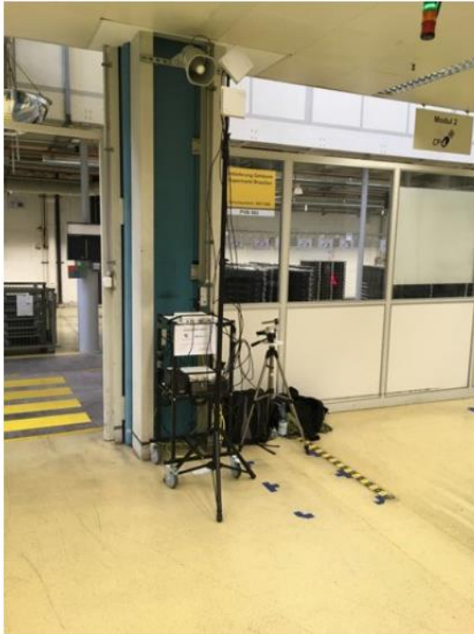
40 deg. directional panel TX @ 2.6m EIRP ~ 23 dBm
