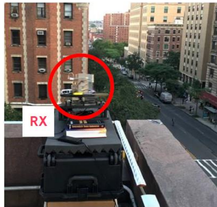
Rx at rooftop, w/o setback from edge
